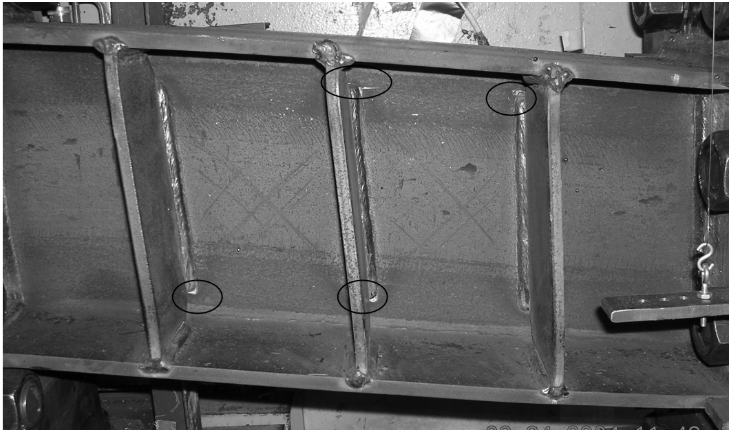
Figure 3.61 Specimen 9: Cracks observed during the first cycle of load step 12 ( \gamma= 0.11 radian)
