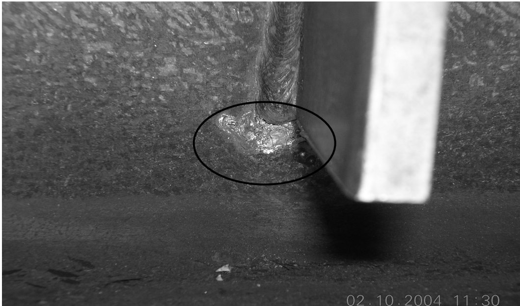
Figure 3.49 Specimen 7: Crack observed at the bottom of the north stiffener after the fourth cycle of load step 7 ( \gamma = -0.05 radian)
