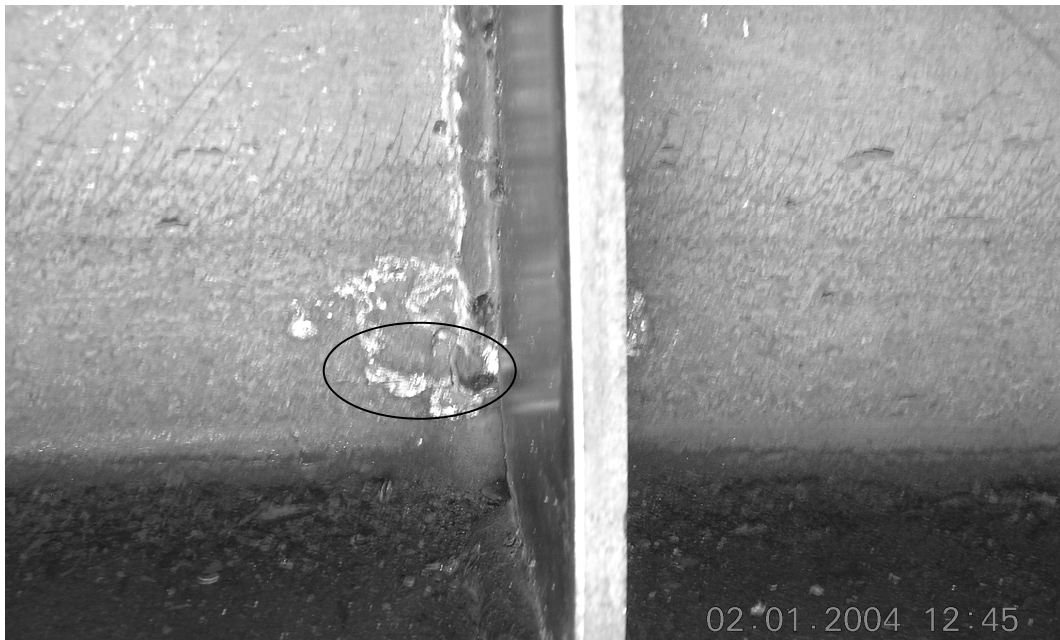
Figure 3.35 Specimen 4: Crack observed after the fourth cycle of load step 8 ( \gamma = -0.06 radian)
