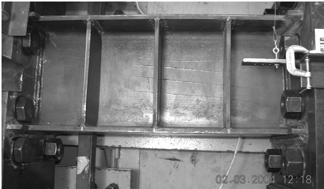
Figure 3.39 Specimen 5: Web yielding after completion of the first cycle of load step 3 ( \gamma = \pm 0.01 radian)
