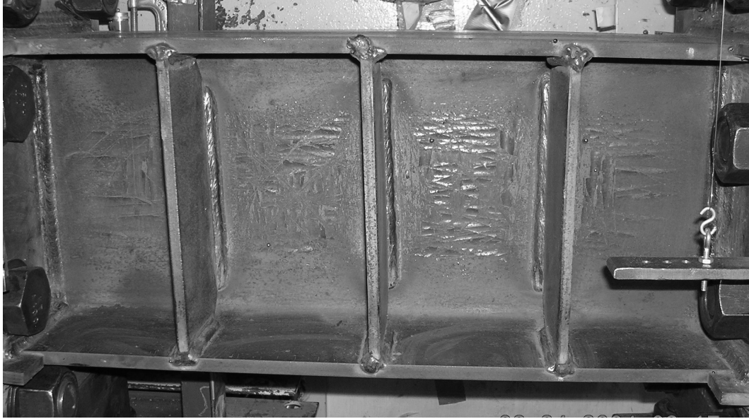
Figure 3.59 Specimen 9: Web yielding during the sixth cycle of load step 4 ( \gamma = -0.01 radian)
