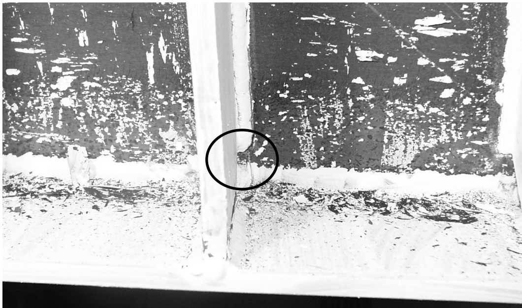
Figure 3.27 Specimen2: First crack observed at the bottom of the center stiffener after the fourth cycle of load step 6 ( \gamma = +0.04 radian)
