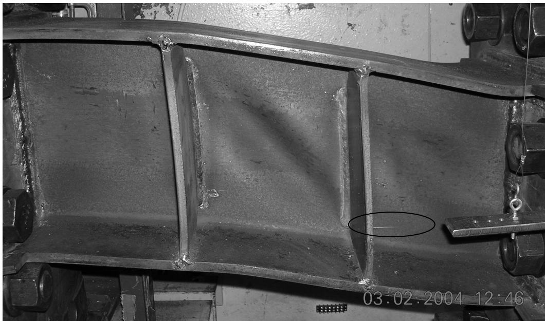
Figure 3.68 Specimen 10: Web buckling and cracks observed after the first cycle of load step 13 ( \gamma = -0.13 radian)
