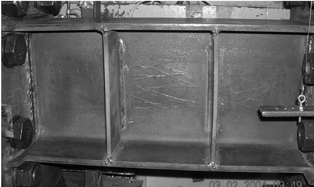
Figure 3.65 Specimen 10: Web yielding observed after the fourth cycle of load step 3 ( \gamma = 0.0075 radian)
